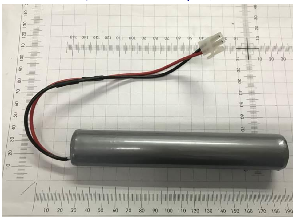
Overall view of battery with enclosure for SP3001bb-ccc (Two 1500 mAh 3.2V battery cells)
