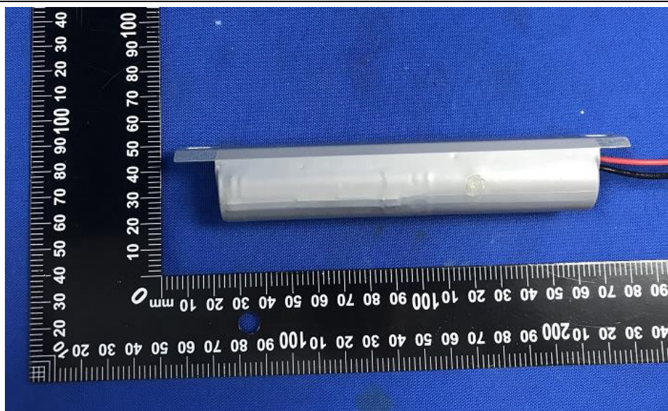
Overall view of battery for SP3002bb-ccc (Two 3200 mAh 3.2V battery cells)
