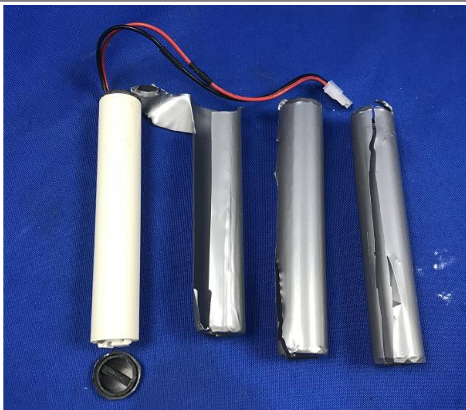
Disassembly view of battery for SP3001bb-ccc (Two 1500 mAh 3.2V battery cells in the enclosure)
