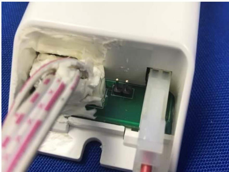
Output terminal without wire link for SPaaaabb-D40
