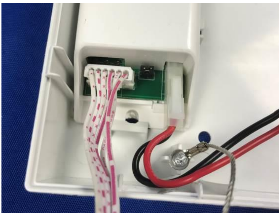
Output terminal of emergency controlgear
