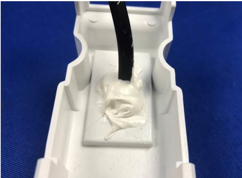
Internal view of cord entry and cord anchorage (fixed by glue)
