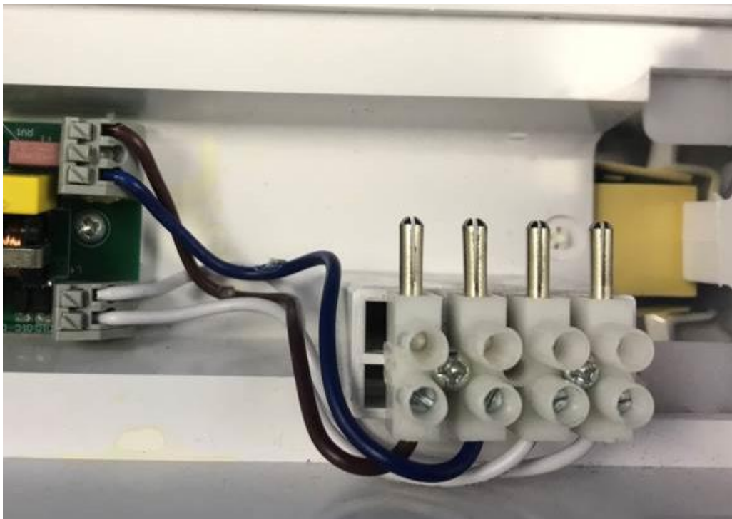
Internal wire connected emergency controlgear and AC connector
