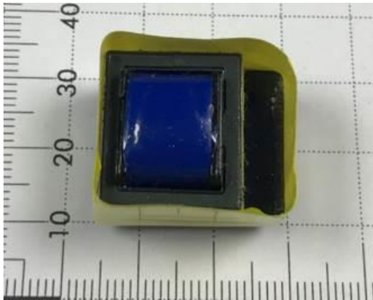
Overall view (the insulation tape wrapped the transformer at least three layers)
