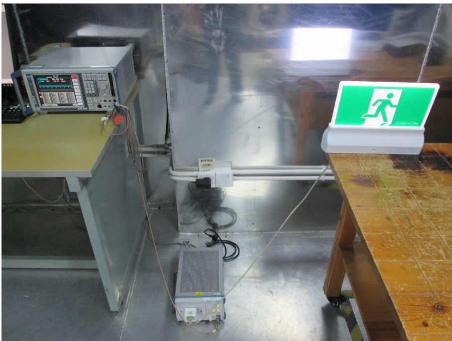
Figure B-2 Setup for Conducted Emission (Emergency)
