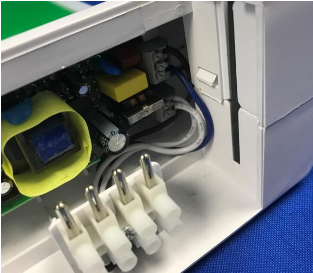
Internal wire (connected emergency controlgear and AC connector)
