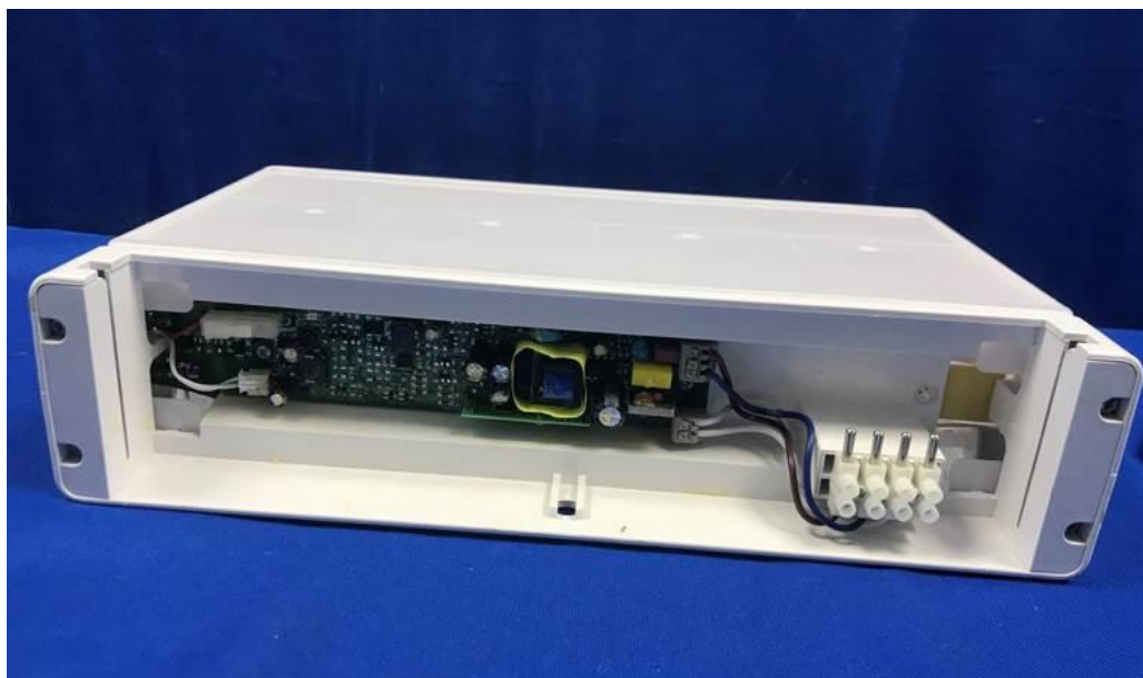
Internal view of SP2001DA-WH
