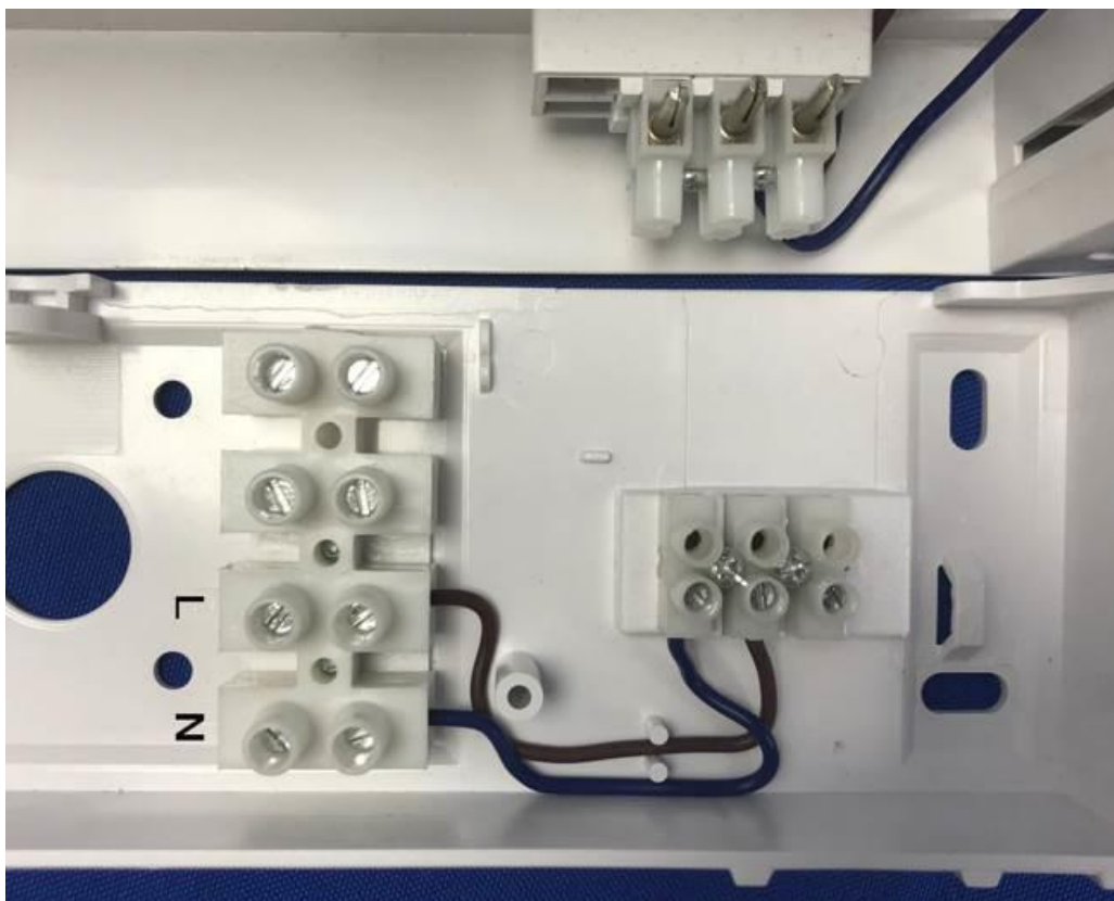
Input terminal block and AC Connector for SPxxxxFE-ZZ series
