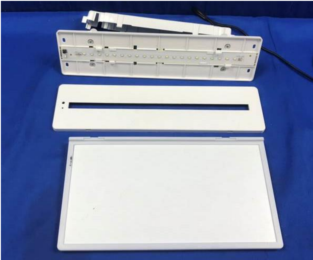
Disassembly view of LED module part
