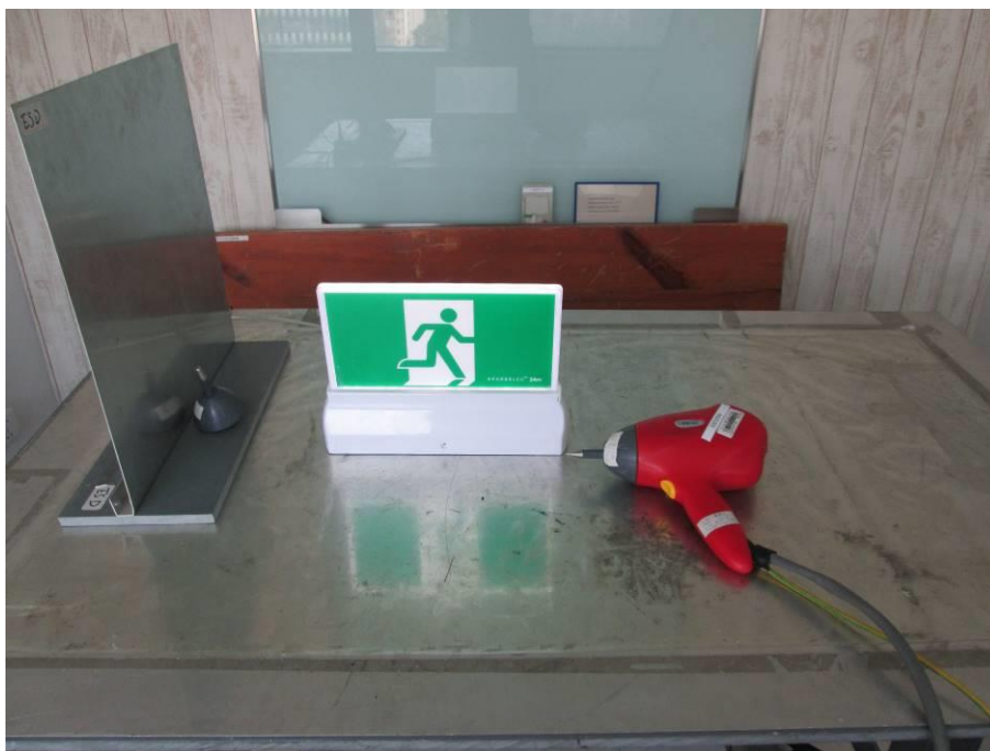
Figure B-7 Setup for Electrostatic Discharge (Charging)
