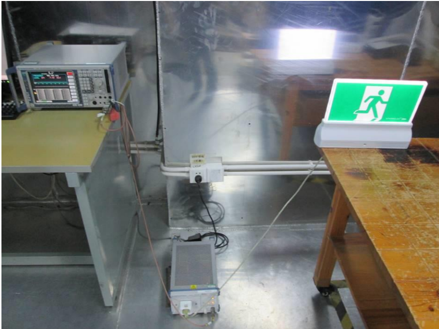
Figure B-1 Setup for Conducted Emission (Charging)
