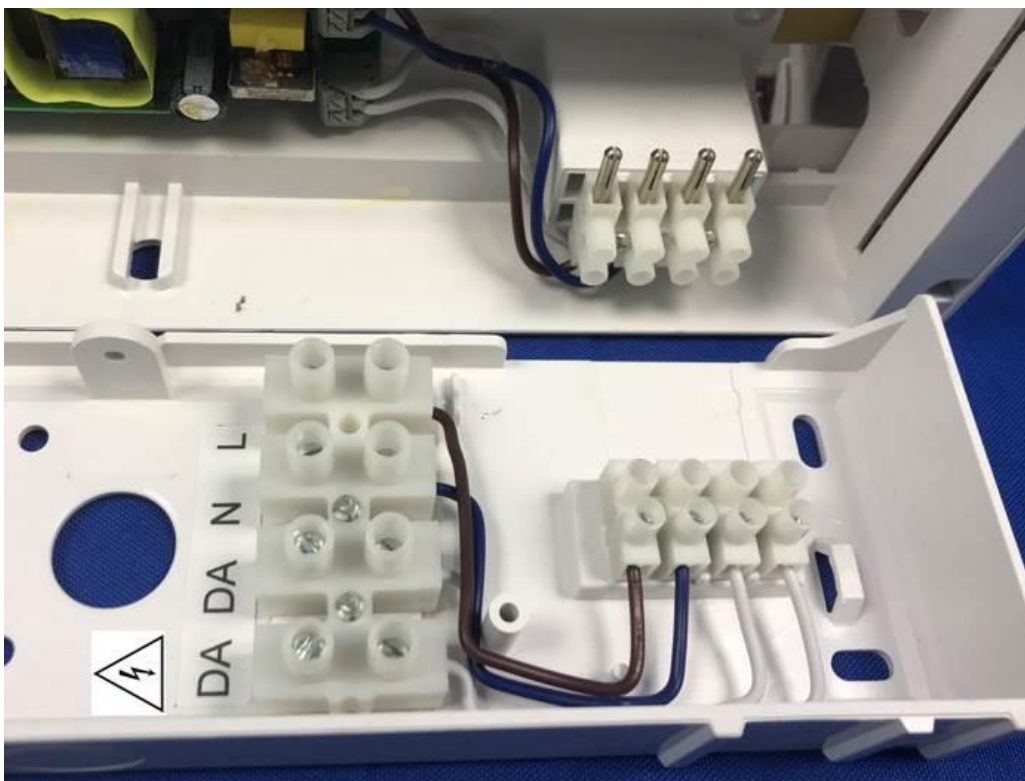
Input terminal block and AC Connector for SPxxxxDA-ZZ series
