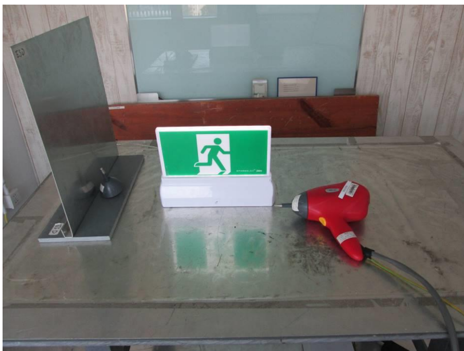
Figure B-8 Setup for Electrostatic Discharge (Emergency)
