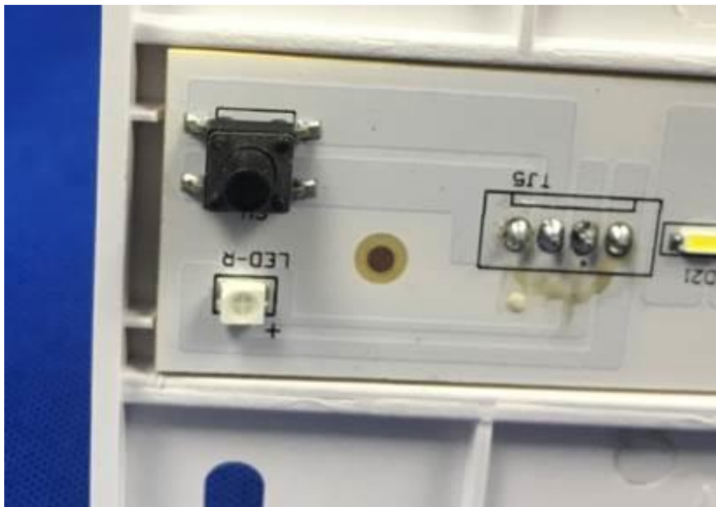
Test switch and LED indicator
