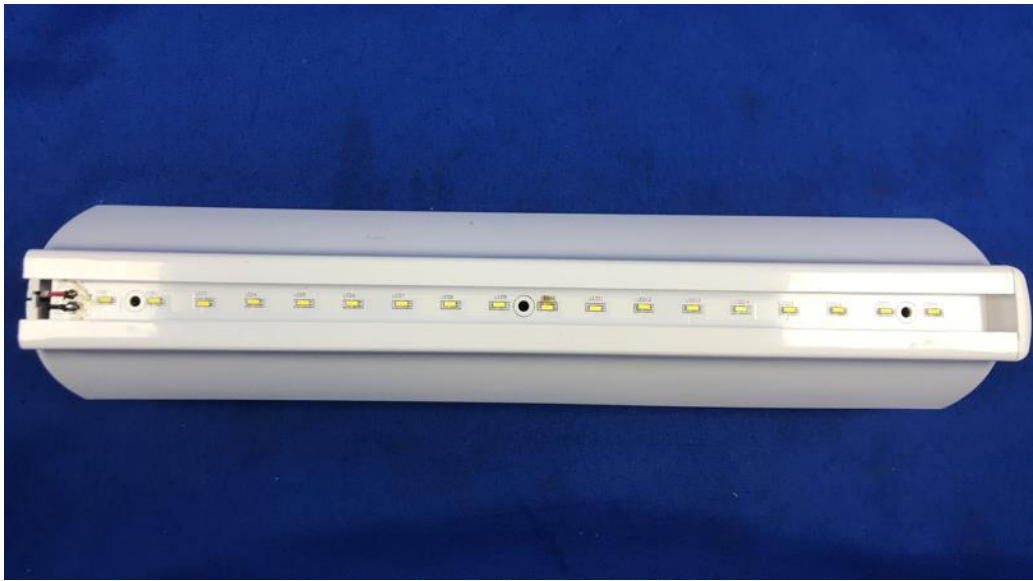
LED module of internal view of SP2003 series
