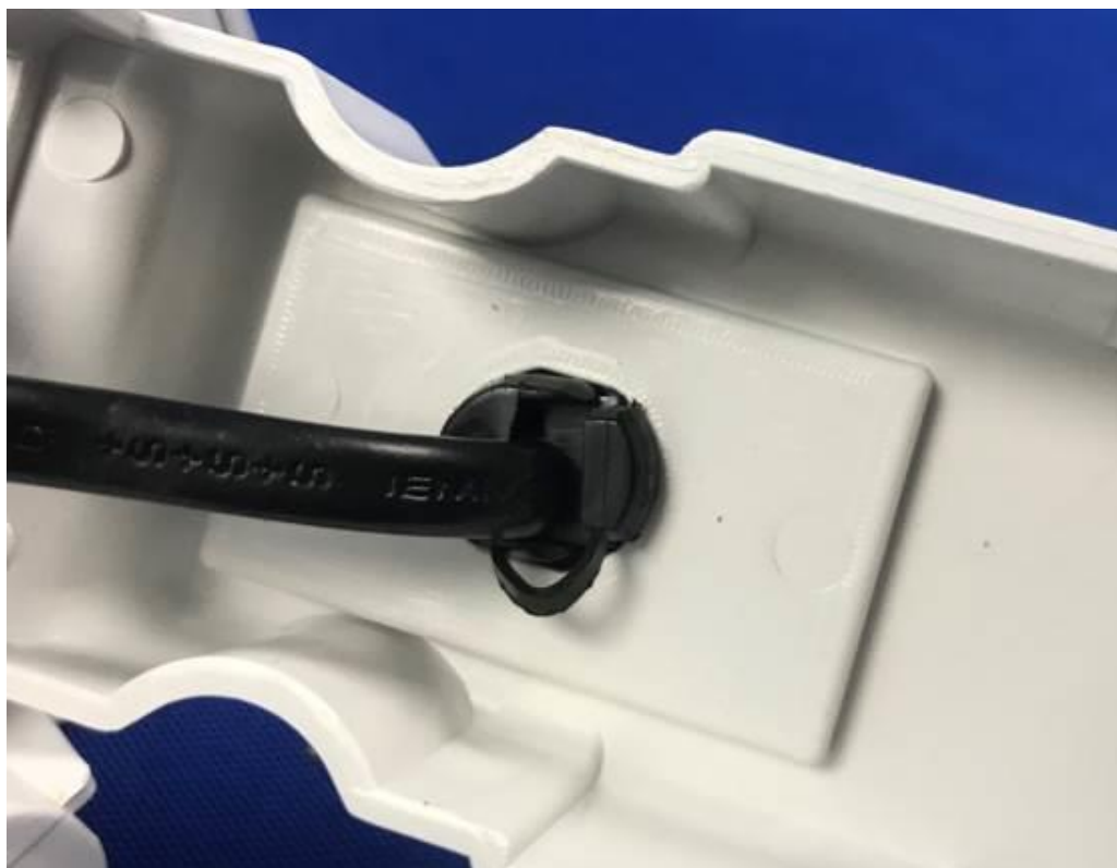
Internal view of cord entry and cord anchorage (removed the glue)
