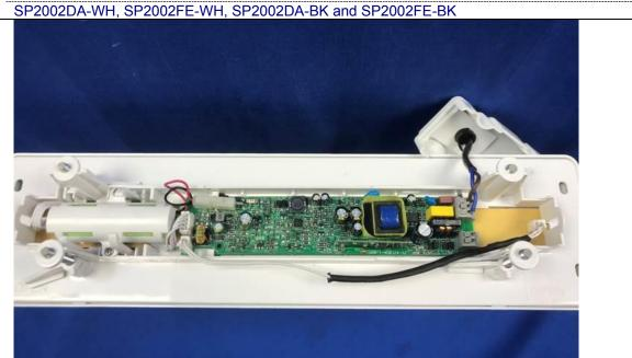
Details of: Internal construction
