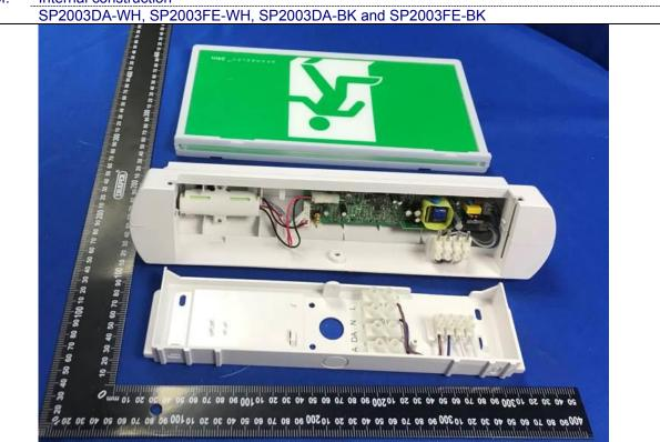
Internal construction Details of:
